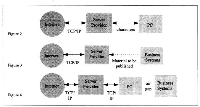
It is fundamental that this model does not provide any other computer systems at the business with direct access to, or from, the Internet. The "air gap" shown in Figure 4 is a critical component in securing the business data from attack by remote access.
